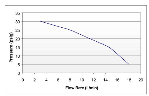
Figure 4 – Zero-Air Generator Performance Curve
