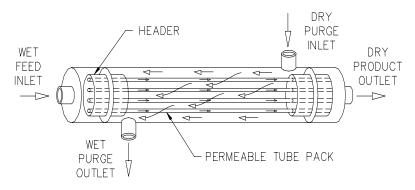
Figure 2 – Perma Pure Nafion Membrane Dryer Schematic
